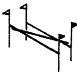
Neither end of cross pole supported by standard cup or fitting
